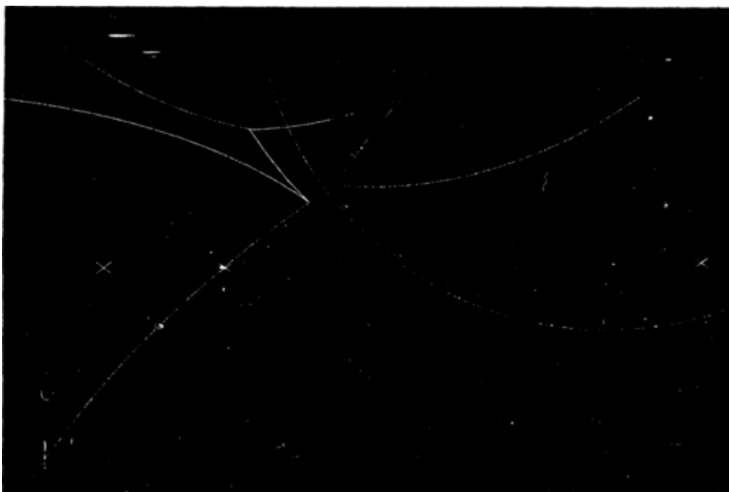
FIGURE 5.2 A proton and an antiproton collide at high energy, producing a couple of almost free quarks.
